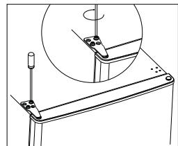
12. Put the hinge cover and the screw cover back.
