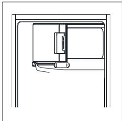
8. Unscrew bottom hinge. Then remove the adjustable feet from both sides.
