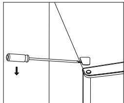
3. Move the core cover from left side to right side. And then lift the upper door and place it on a padded surface to prevent it from scratching.
