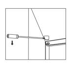
4. Move the core cover from left side to right side. And then lift the upper door and place it on a padded surface to prevent it from scratching.
