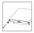
11. Install the upper door with the upper hinge.
