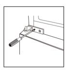
10. Unscrew right middle stopper with metal block from bottom of upper door. And then install left middle stopper and metal block in left side of bottom of upper door.
