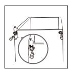
9. Make the middle hinge reverse the direction 180°C, then transfer it to the left property position.
